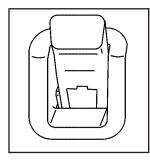
From the inside, use the manual lock levers located on the door panels near the windows. **Central Door Unlocking System**
